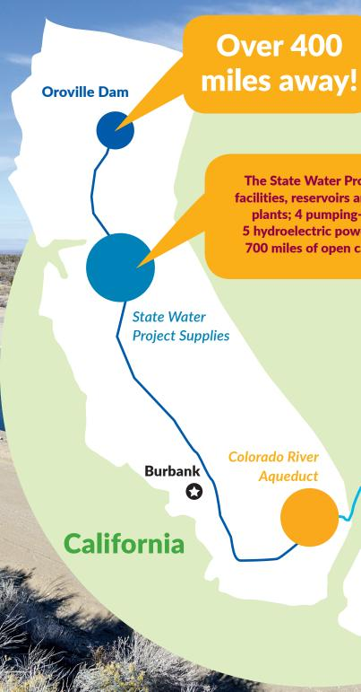
The State Water Project has 34 storage facilities, reservoirs and lakes; 20 pumping plants; 4 pumping-generating plants; **5 hydroelectric power plants; and about** 700 miles of open canals and pipelines.
